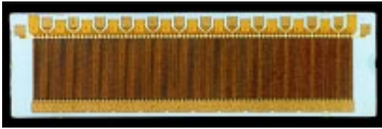
Fig.2 Top view of FET chip (chip size = 1.1mm x 3.6mm)
